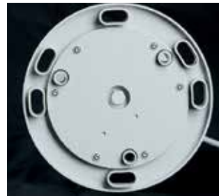
Installation The bottom plate of the SC 110 supports installation on structure using 3 or 4 x M12 on a 200 mm diameter or 3 x M8 on a 150 mm diameter.
